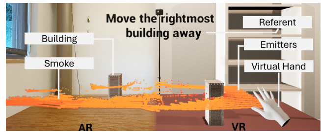
Figure 3: The view the participant sees during the study. The left half is the AR environment, while the right half is the VR environment. The environments include a building, emitters, smoke, and, for the VR scenario, a virtual hand inside the virtual environment.
